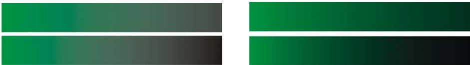
Figure 12: CMYK Black is added (left). Color 100C100M100Y100K is added (right).
