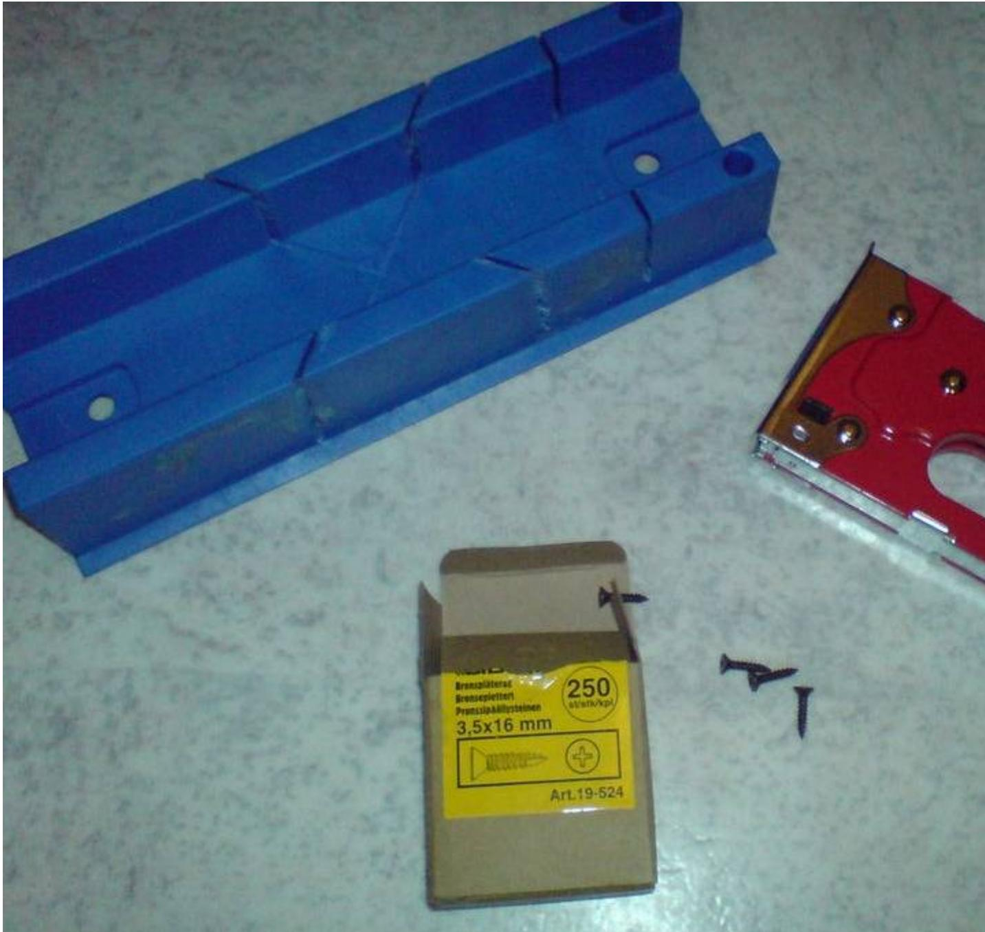
First thing to do is to build the frame. I went to the lumber yard and got regular unfinished lumber (40mm x 30mm) to make the inner frame. I also got some finished wood to use as the outer frame. You also need some L brackets, wood screws, a staple gun and a miter box (if possible though, use one of those miter saws that are attached for better precision).
