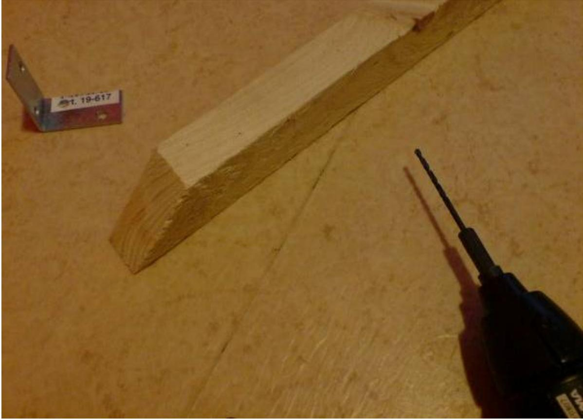
Now it's time to make the inner frame. Just saw the unfinished lumber to make a rectangle of 16x9 proportions (I made miter joints but it's probably easier and better to make regular joints since these won't show anyway). To ensure the structural integrity of the thing I also put a cross in the middle.
