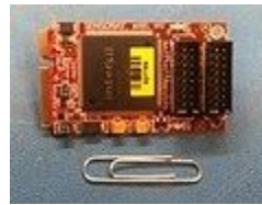
A Mini PCIe card that simultaneously captures 8 video and 8 audio signals (Sensoray 1012)
